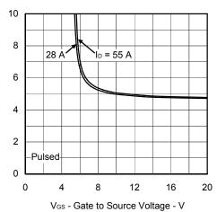
RDS(ση) - Drain to Source On-state Resistance - mΩ
